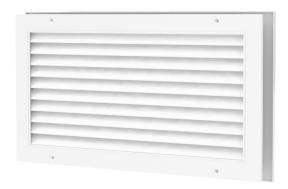
Grille for transfer air between rooms. Installed in door or wall. Installation thickness for grille and frame is 25-50 mm. If wall or door thickness exceeds 50 mm, two grilles can be used without mounting frame. Airflow through the grille is caused by pressure difference between rooms.
