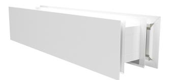
Airflow through the grille is caused by pressure difference between rooms. The grille includes sound absorbing plates to attenuate sound between rooms and absorb air flow noise.
