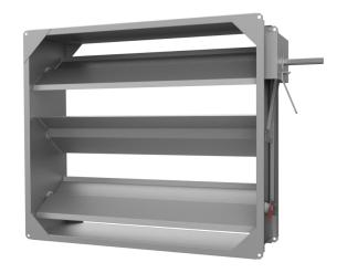
KR4-S - Edge-sealed damper for shut-off and regulation with thermal insulation, tightness class 3 (EVS-EN 1751:2014). For systems with high temperature variations and high requirements for tightness. KR4-S the measured thermal transmittance  $U_m=4 \text{ W/m}^2\text{K}$ .
