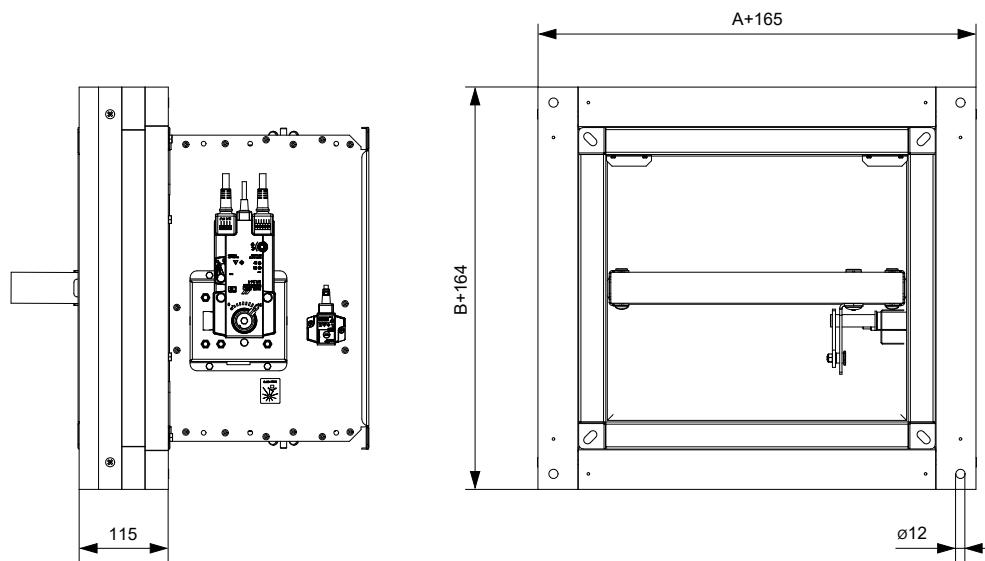
Fig. 47. In solid wall construction - installation frame E4
