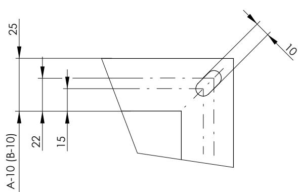
20 mm wide flanges are fitted with oval holes in the corners.
