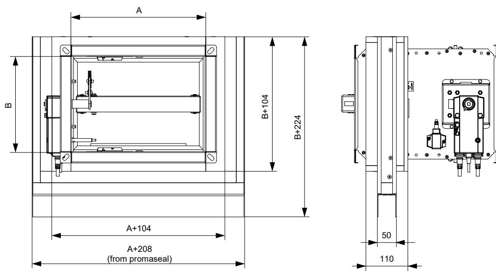
Fig. 50. In solid ceiling construction – installation frame E5
