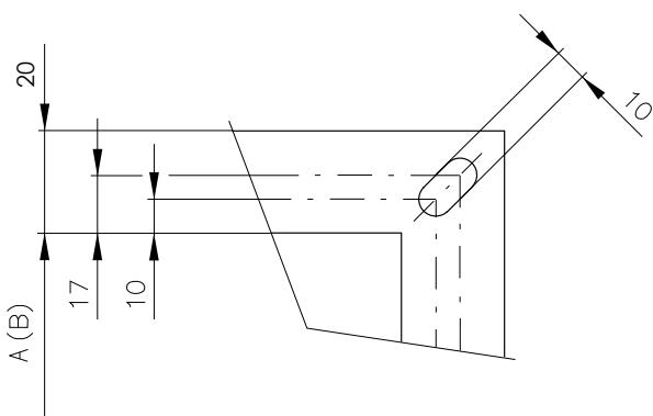
Fig. 11. Flange of Damper - INSTALLATION SIDE
