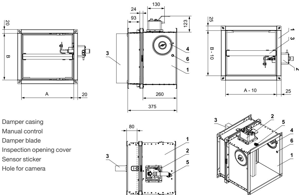
Fig. 8. FDMQ with spring return actuator
