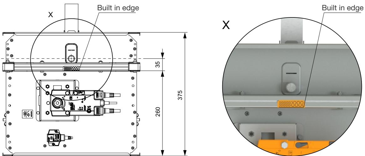
The damper must be installed so that the entire damper blade - in the closed position - is located inside the fire separating structure (wall) and at the same time the control mechanism and inspection openings are freely accessible. „Built in edge label” indicates the “maximum“ edge of installation of fire damper into the fire partition structure.
