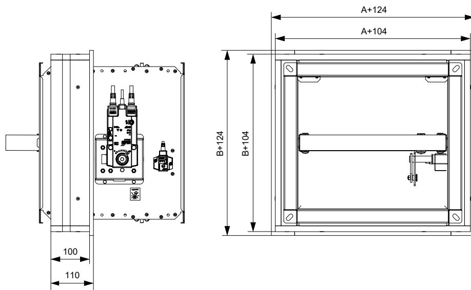
Fig. 41. In solid wall construction - installation frame E1
