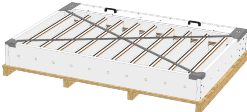
2. Place handling inserts between the top slat and the damper housing.
