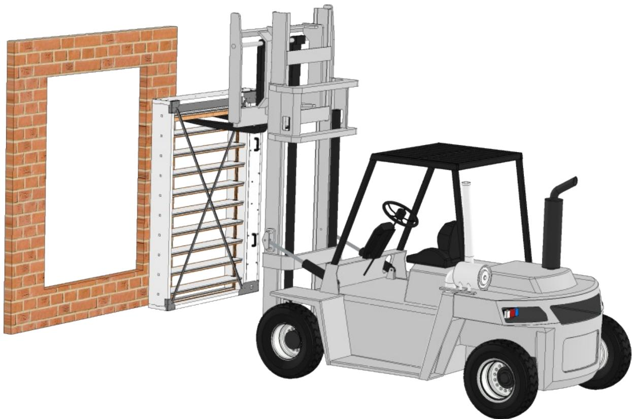
5. After installing the damper and possibly hardening the plaster/mortar, remove the transport struts and corners.
