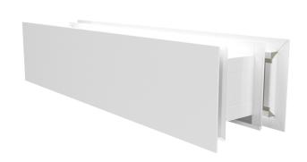
Airflow through the grille is caused by pressure difference between rooms. The grille includes sound absorbing plates (made of synthetic material) to attenuate sound between rooms and absorb air flow noise.
