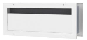
Installing thickness 95-135 mm. Airflow through the grille is caused by pressure difference between rooms. The grille includes sound absorbing plates to attenuate sound between rooms and absorb airflow noise. Usually installed in wall above a door.
