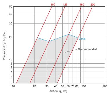
The air intake grille should be selected in such a way that the air velocity at the intake does not exceed 2 m/s.
