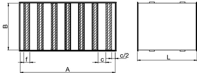
**MSK/MSC sound attenuation (absorption material mineral wool)**
