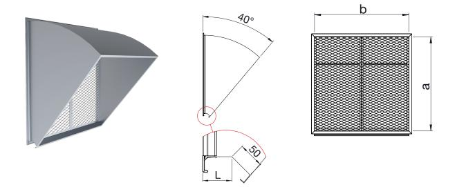
EVR is a diagonal air intake with mesh is suitable for use at the end of both the supply and exhaust duct. Dimensions a, b ( $\leq$  2500) are nominal sizes.
