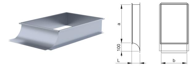
Flat saddle for a rectangular duct. One edge of the saddle is provided with a connection bar and larger end with flange for riveting into duct side. Standard length is 125 mm.
