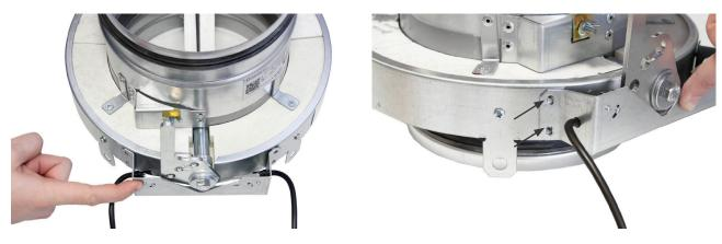
3. Adjust and tighten the limit switch to the position so that the switch goes to the bottom in both positions and that there is a click heard in the end.
