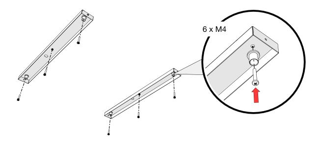
ATTN! Choose appropriate fastening devices depending on the ceiling type Diameter of the mounting holes in the ceiling bracket are 4.5mm.
