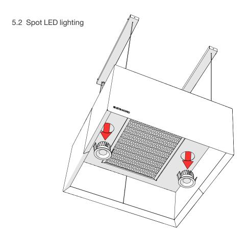
Spot LED lighting is fastened with spring clips on the top surface of the canopy ceiling. For replacing the luminaire, it should be pulled downward from the canopy ceiling.
