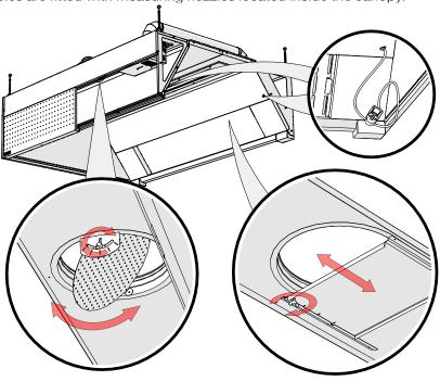
ATTN! During measurement, HFK all grease filters and blind plates must be in place and the front panel must be closed.
