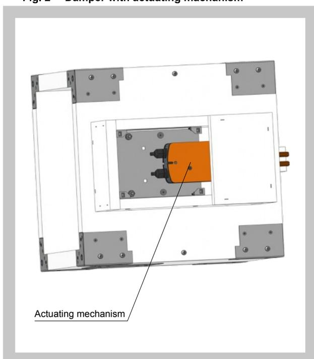
Tab. 2.1.1. Actuating mechanism BELIMO BLE 24(-ST), BLE 230
