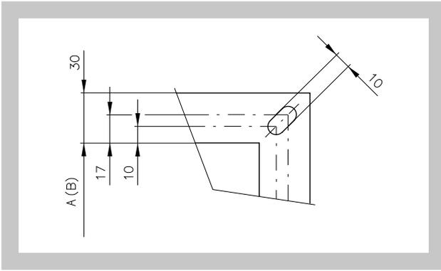
4.3. For damper without flanges (Fig. 15) the open damper blade overlaps the damper body from dimension B = 250 by the value "c" or "a" and "c". These values are specified in the Tab. 4.2.1.
