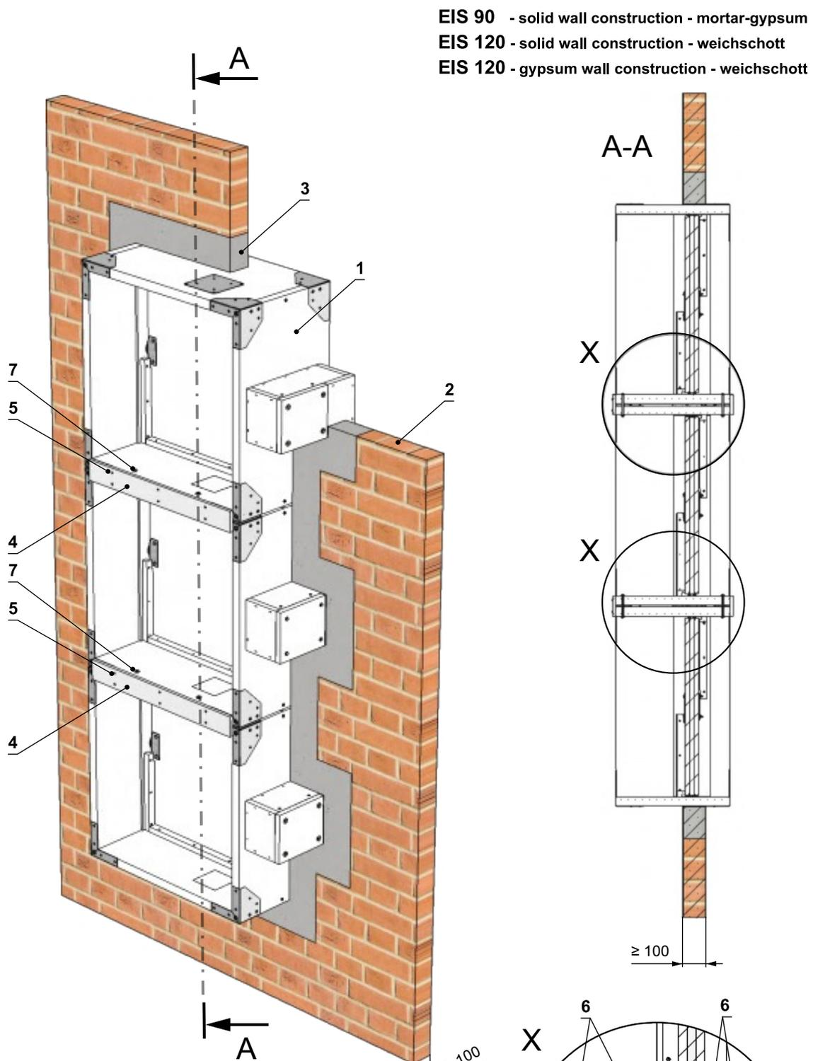
EIS 90 - solid wall construction - mortar-gypsum
