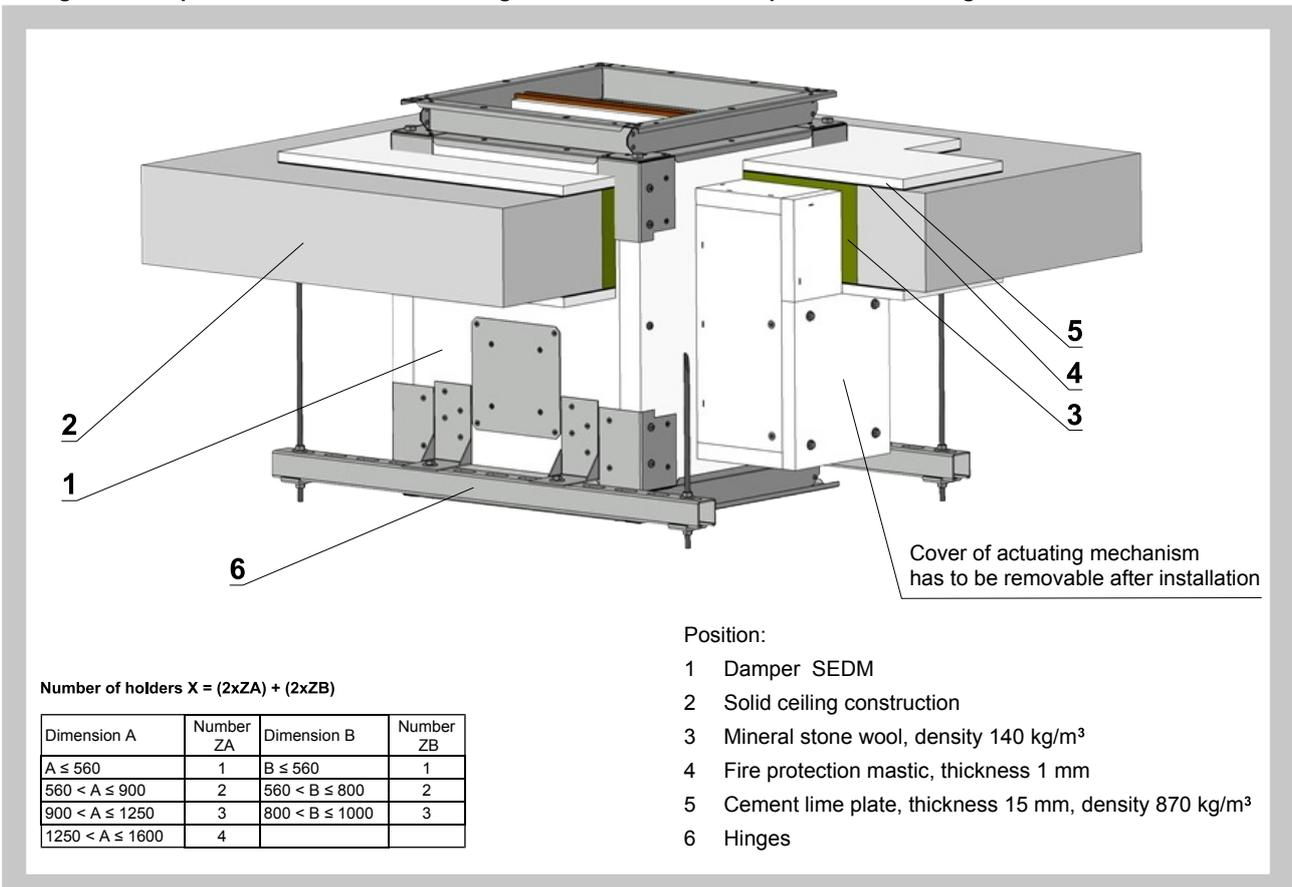
Fig. 24 Example of installation in solid ceiling construction of fire compartment - actuating mechanism above
