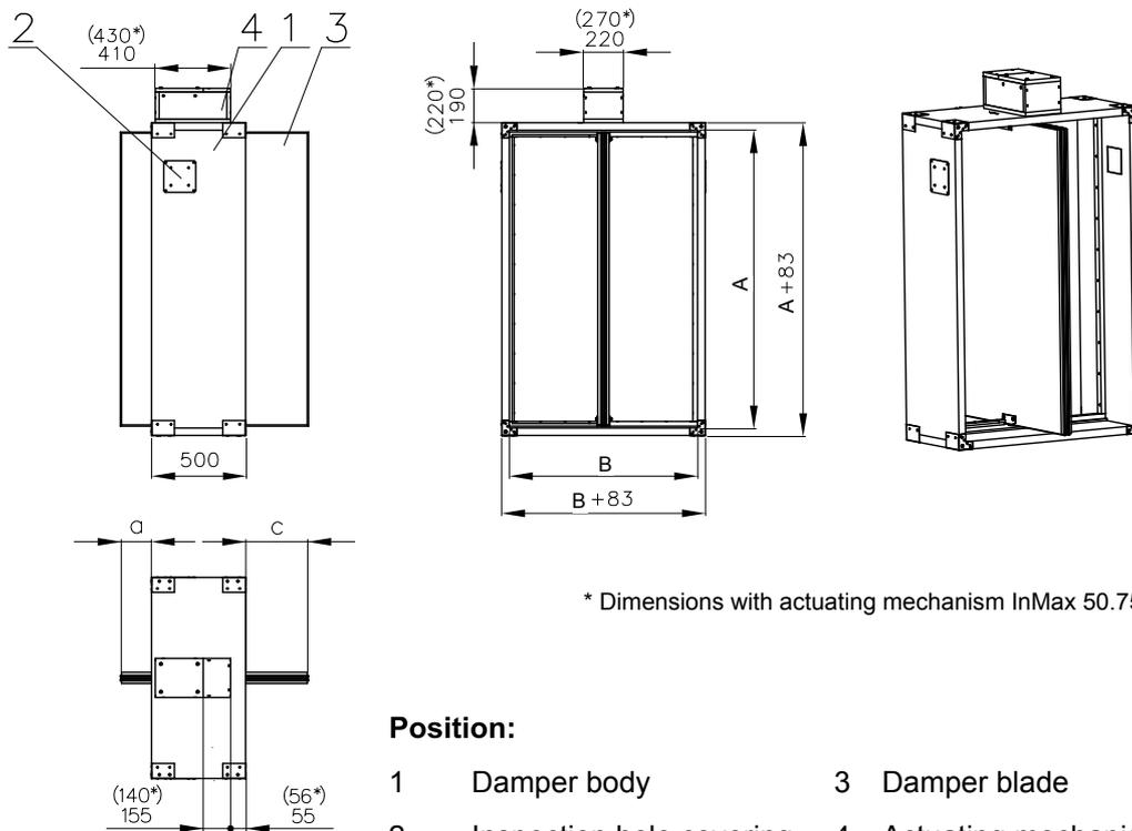
Fig. 12 Smoke extraction dampers - multi with flanges
