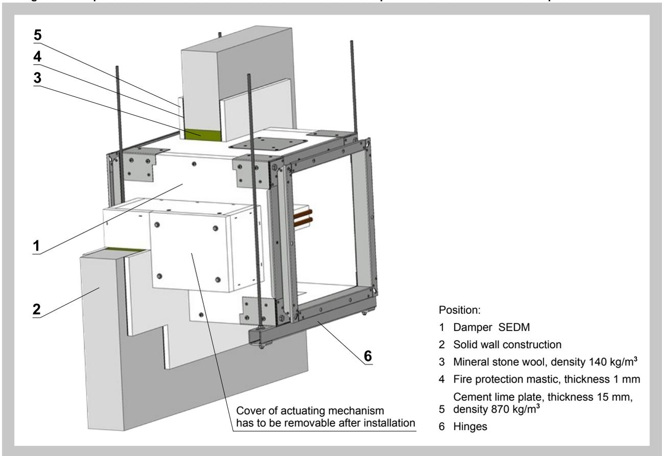
Fig. 19 Example of installation in solid wall construction of fire compartment - vertical blade axis position.
