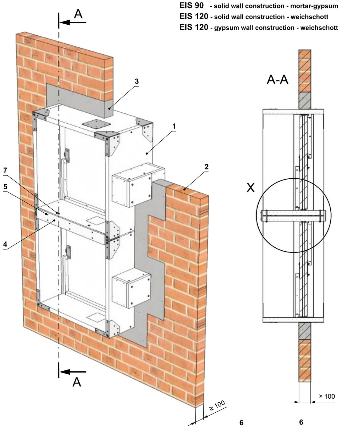
EIS 90 - solid wall construction - mortar-gypsum
