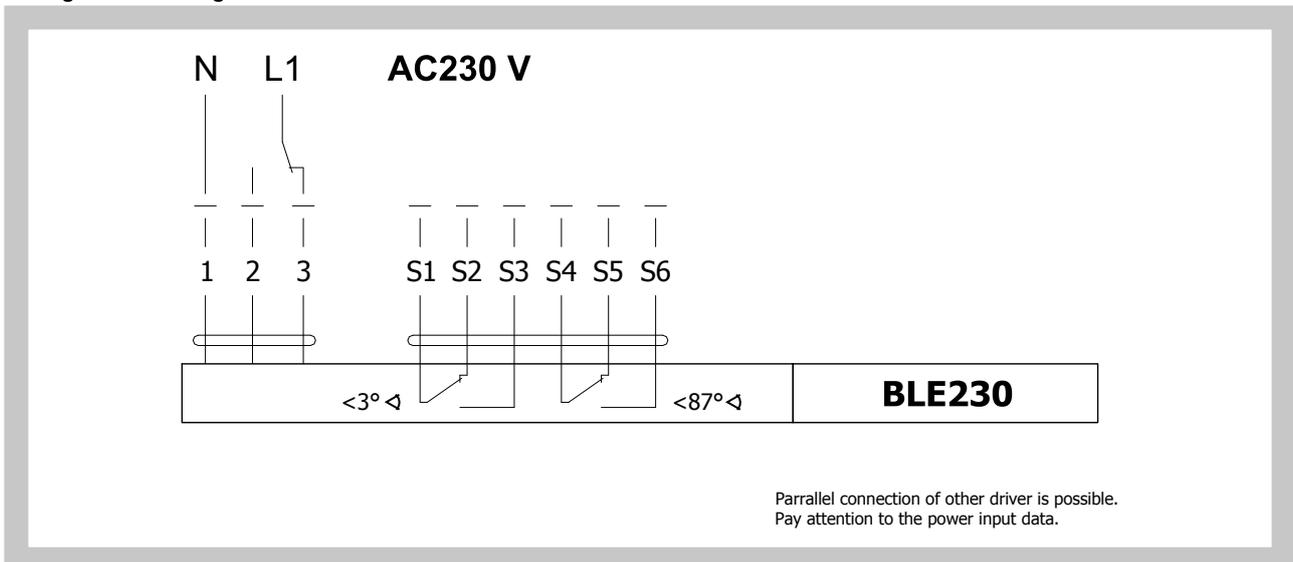
Tab. 2.1.2. Actuating mechanism BELIMO BE 24-12(-ST), BE 230-12
