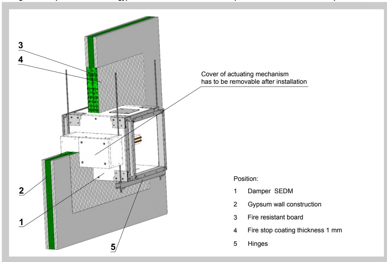
5.4.3. Installation on solid wall or ceiling construction of fire compartment
