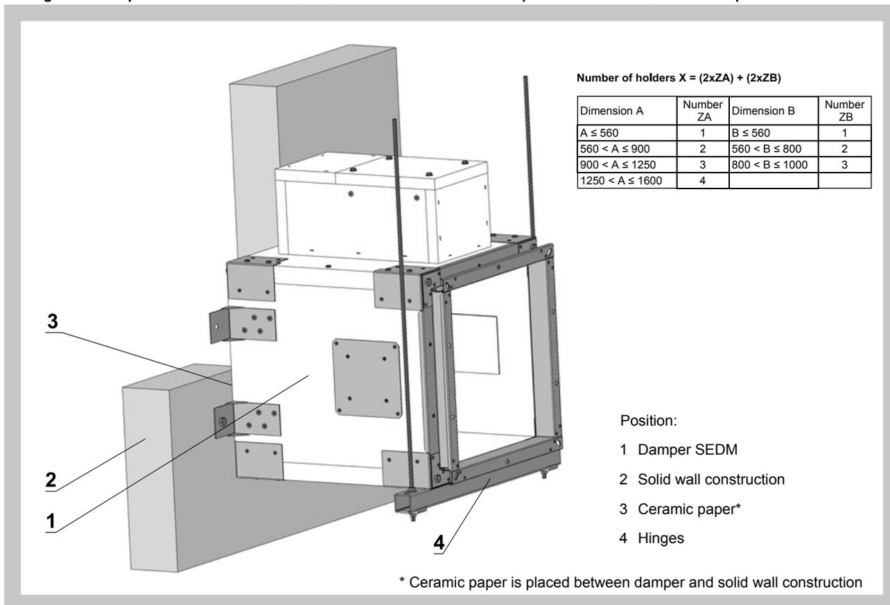
Fig. 34 Example of installation on solid wall construction of fire compartment - horizontal blade axis position.
