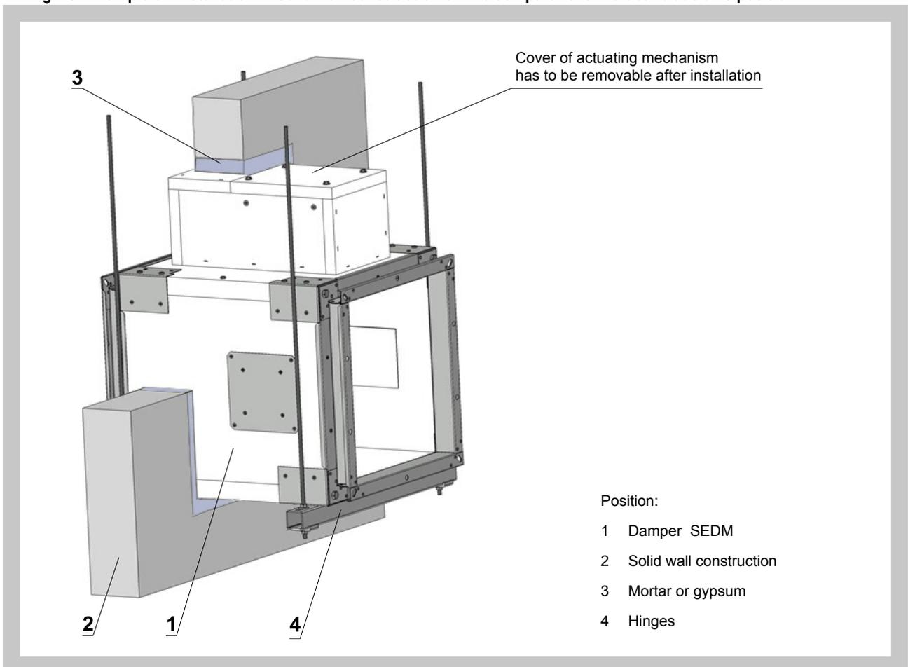
Fig. 20 Example of installation in solid wall construction of fire compartment - horizontal blade axis position.
